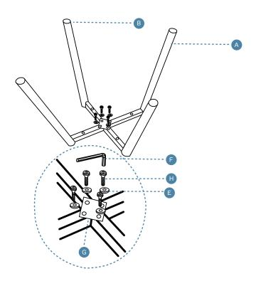
Attach 1 x leg (A) and 1 x leg (B) together as shown and secure with 1 x plate (G),  $4 \times 10^{-2}$  x bolts (H) and  $4 \times 10^{-2}$  washers (E). Tighten with an Allen Key (F).
