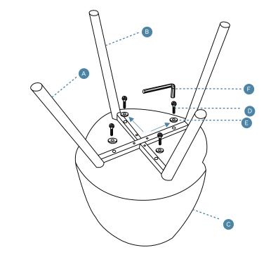
Attach assembled frame to chair as shown and secure with 4 x bolts (D) and 4 x washers (E). Tighten with an Allen Key (F).
